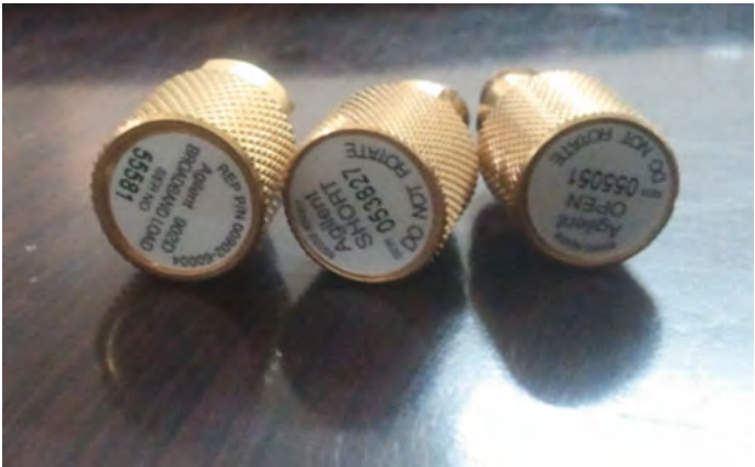
Fig. 12.51 Short, open, and load termination for calibration of VNA
