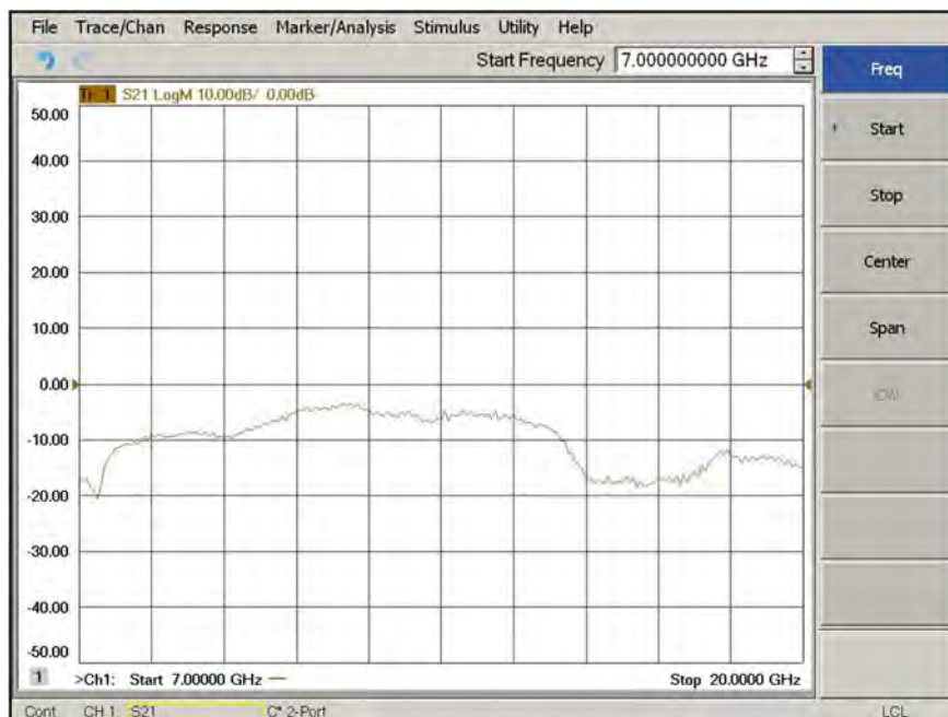
Fig. 12.38 S21 measurement plot in dual feed of simulated DRA
