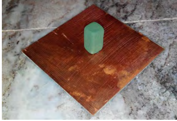
Fig. 5.1 Homogenous dielectric RDRA on ground plane
