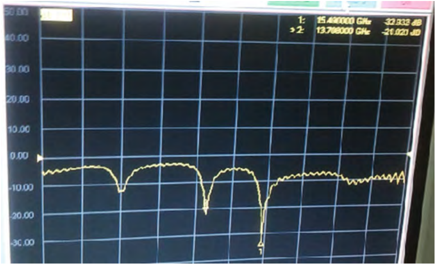
Fig. 12.59 VNA showing measured S11 of RDRA
