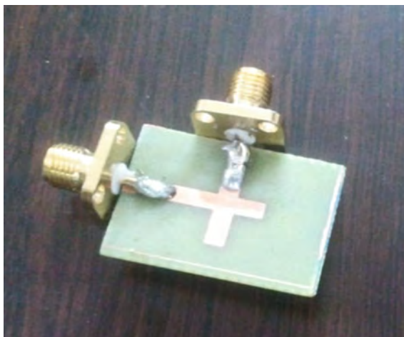
Fig. 12.52 Top and side view of single- and double-feed aperture couple feed of RDRA
