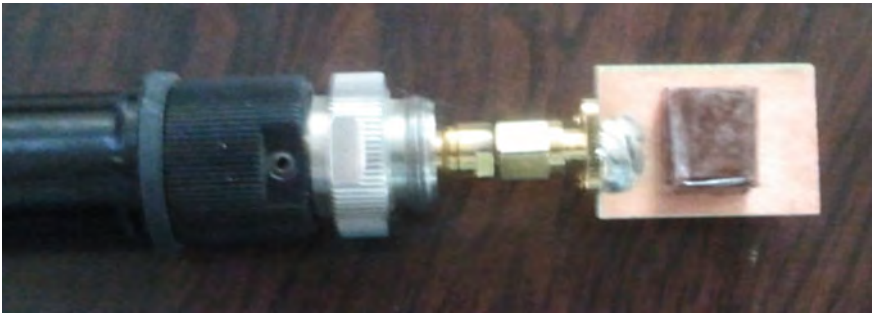
Fig. 12.60 Fabricated model of RDRA under test with single feed and slot
