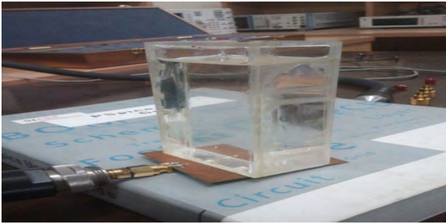
Fig. 8.8 RDRA under measurements with VNA
