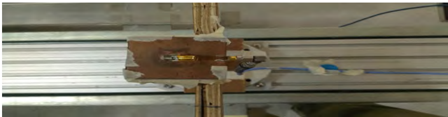
Fig. 12.2 Positioning of RDRA antenna ready for test procedure setup
