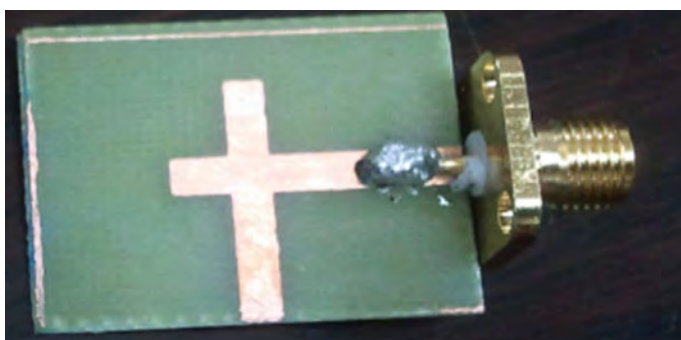
Fig. 12.63 Top view with single feed and SMA connector of fabricated RDRA
