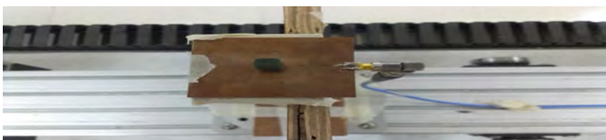
Fig. 12.6 View of RDRA antenna under test setup on sliding table
