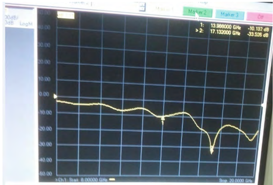
Fig. 12.18 Measured return loss S11 at -33.596 dB of RDRA
