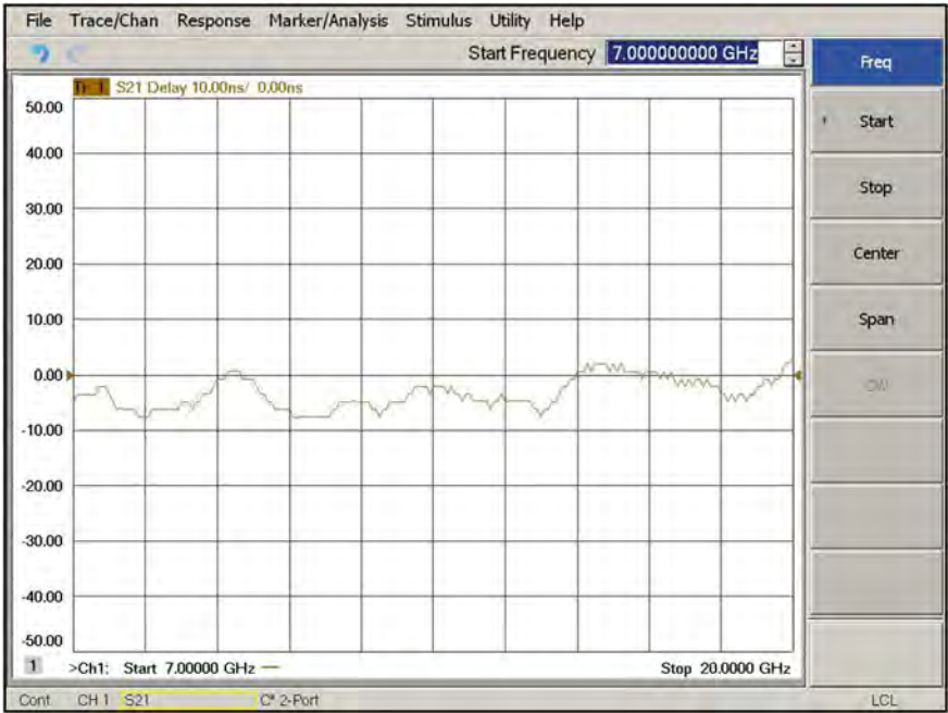
Fig. 12.36 Group delay measurements in RDRA dual feed of simulated DRA
