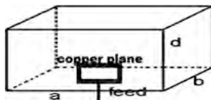
Fig. 10.1 RDRA with copper x, y rectangular plane and feed d length
