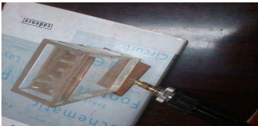
Fig. 8.13 Measurements of RDRA with aspect ratio changed
