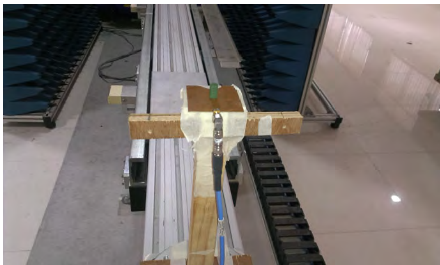
Fig. 7.31 RDRA mounted with wooden block for measurement
